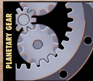
The multiple gears found in planetary gear winches translate to greater pulling speed.
