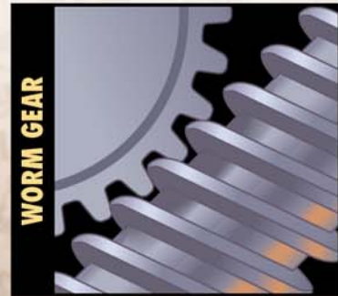
Consisting of a cylindrical worm and a typical round gear, worm gear winches offer brute strength.
